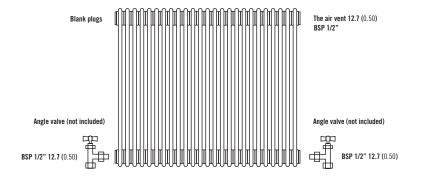
Note: Factory fitted bushes are welded in place and not removable. If installing TBOE (Top Bottom Opposite End) please note that the radiator MUST be inverted.
