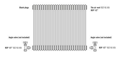
Note: Factory fitted bushes are welded in place and not removable. If installing TBOE (Top Bottom Opposite End) please note that the radiator MUST be inverted.
