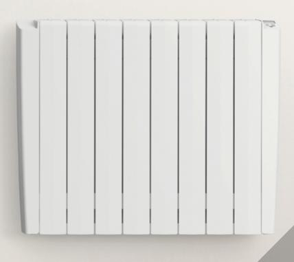
ALU SIMPLE FLUID The Alu Simple Fluid is an oil filled radiator made with slimline and compact vertical flat, double aspect tubes. The Alu Simple Fluid heats up by using an electrical element immersed in thermodynamic oil within the radiator. This maintenance free and specially formulated fluid is designed to distribute the heat quickly and evenly across the radiator, which in turn emits the heat into your room through radiation.
